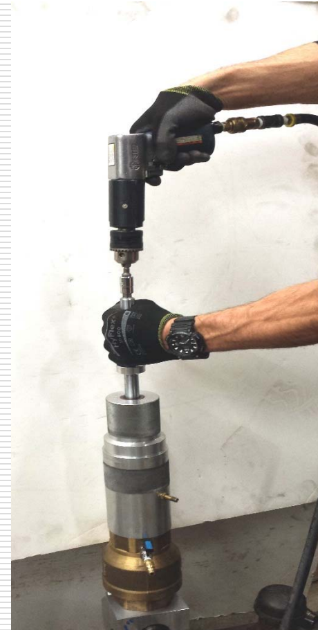
Drill through the backside of the elbow.
