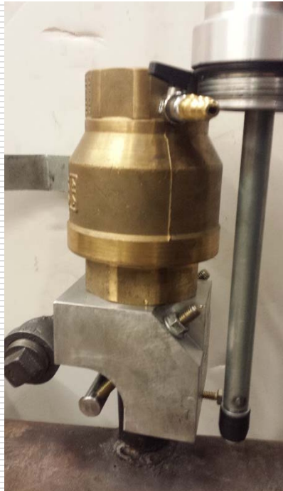
Insert rubber stopper below the branch. (Stopper shown next to housing for illustration)
