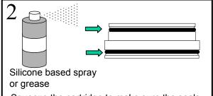
Squeeze the cartridge to make sure the seals expand easily. Lubricate the seals if necessary. Silicone spray or silicone based grease (e.g. Molykote) is preferred.
