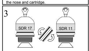
Place the cartridge back on top of the grippers with the required size downward.
