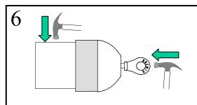
To remove the towing head unscrew the eyebolt.
