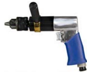
500 rpm geared air drill Common air drills with a single gear drive run at 2000 - 3000 rpm free air speed. These will not have enough power to mix the sealant, especially in cold weather.
