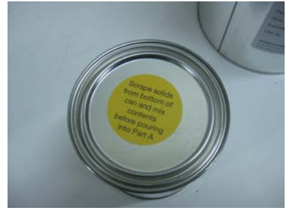
Scrape any solids from the bottom of the Part B can and mix with the paint paddle.
