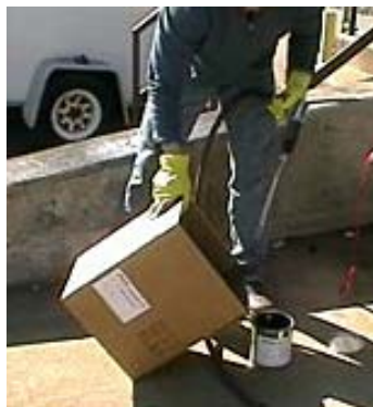
Stop the mixer before removing from the can and spin the mixer head inside an empty carton to remove most of the sealant. Remove the cured sealant from the mixer with a knife each morning.
