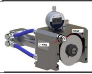
8. Attach dead-man control to air motor. Depress dead-man control and adjust lubricator to 1 drip per second.
