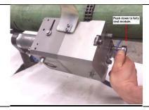
Depress lever on dead-man control to start blade. Turn blade feed knob until blade slightly touches / kisses pipe and release dead-man control.
