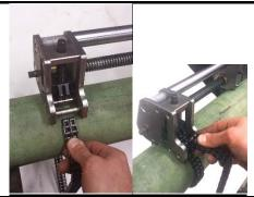
**4.** Move bracket to the desired position. Make sure bracket feet are touching pipe and rail is straight. Tighten chain hooks with small ratchet in an alternating sequence. Do not over-tighten.
