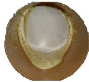
B.) At full expansion, some foam seeps through to seal the pipe.
