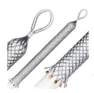
Also known as Towing Socks, Chinese Fingers or Pulling Grips used to pull pipe above or below ground. The harder the pull, the tighter the grip. Commonly used to install pipe or conduit using directional drilling rig (HDD) or vibratory plow.
