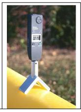
On pipe > 2" position tool on pipe as shown above. On pipe < 2" rotate the tool 90° & position on pipe using the small "V" slot.
