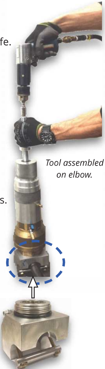
Clamp-on housing provides seal and rock steady base.
