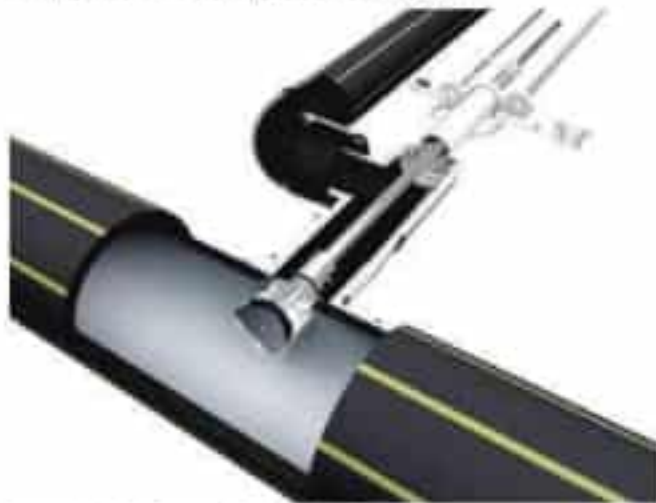
Figure 4— Cutter Tapping PE Main Under Pressure
